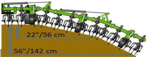
The frame can flex down 15 degrees per section (unlimited up flex). This lets the implement run over or along terraces while maintaining accurate working depth.
