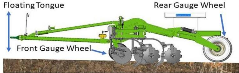
Working depth on the Elxir™ is measured off the front and rear gauge wheels. Combined with the floating tongue this feature enables the unit to maintain front to back depth on peaks and in valleys.
